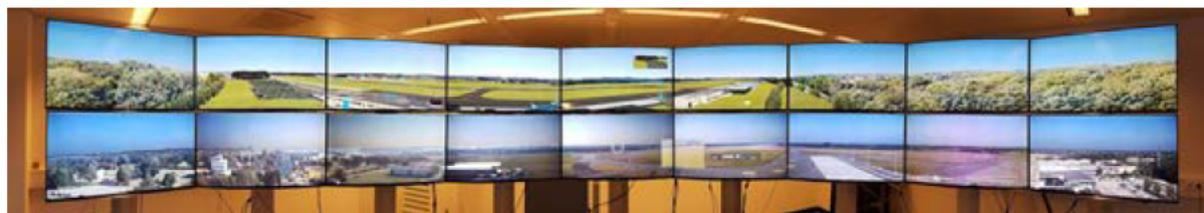
Figure 35: Multiple Remote Tower operation set-up with NARSIM simulation on top
